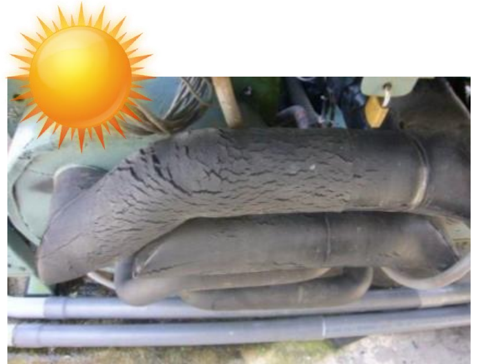
UV damage Rubber
