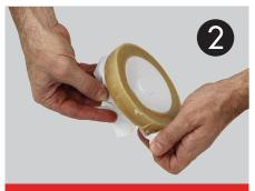
Remove wax seal from plastic mould.
